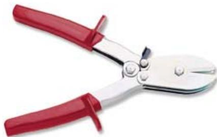
The blades inter-penetrate to form a fold on the periphery of the pipe, reducing its diameter, and allowing consistent slotted joints to be easily formed in all types of pipe (smoke and gas, extraction, ventilation, dust extraction, rainwater downpipes, etc.) Accurate adjustment is obtained by varying the pressure on the handles. - Insulating polypropylene grips. - Case-hardened blades and pins.
